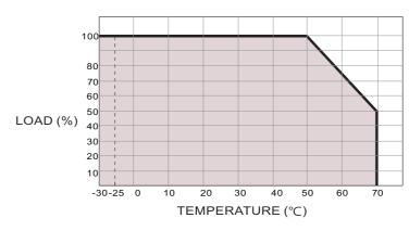
At 84-264VAC input voltage operation, the output load should be as per mention derating curve graph.
